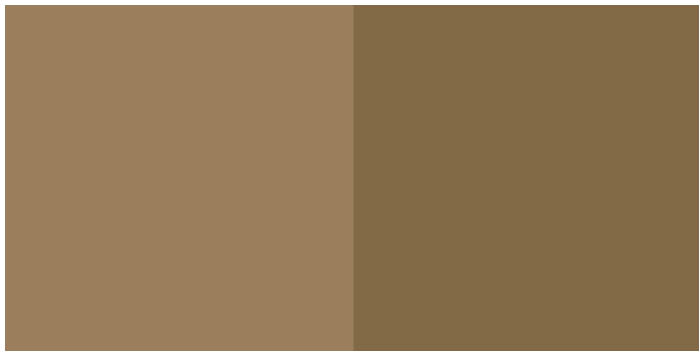
Before & after 12 hours of ammonia fuming. Colours sampled in Photoshop from same location on offcut.
