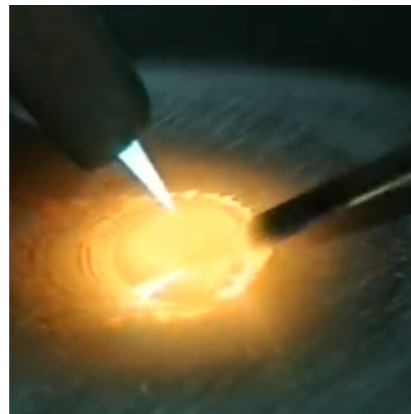
Perfect puddle, flame tip distance and filler rod dip location.
